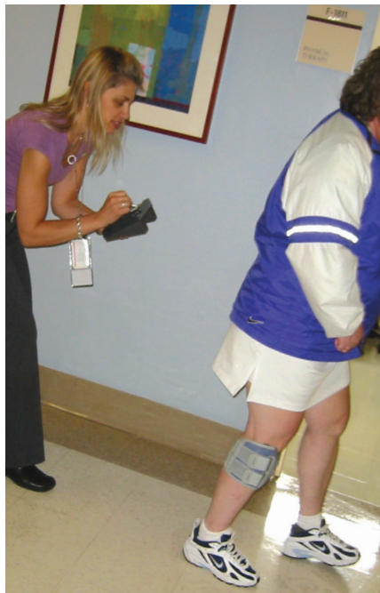
Gina Sauro, PT, uses wireless technology to fine tune the stimulation parameters on the L300 functional electrical stimulation device.
